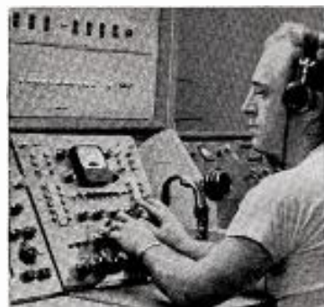
An interim General Electric 100-watt transmitter powers the WEEU-TV signal to Reading and Berks County.
